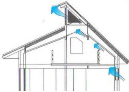
Figure 4: Natural air convection in a system that includes angled ceiling, solar blind and clerestory is an application of the Venturi and Bernoulli effects at CasaE-UFRGS.
