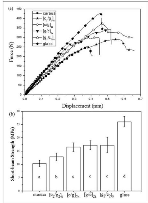
**Figure 4.** Typical short-beam curves of the laminates (a) and mean inter-laminar shear strength of the composites (b).
