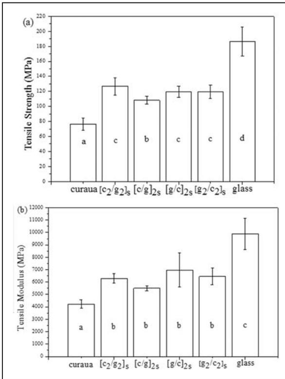
**Figure 3.** Mean values of tensile strength (a) and modulus (b) of the laminates.
