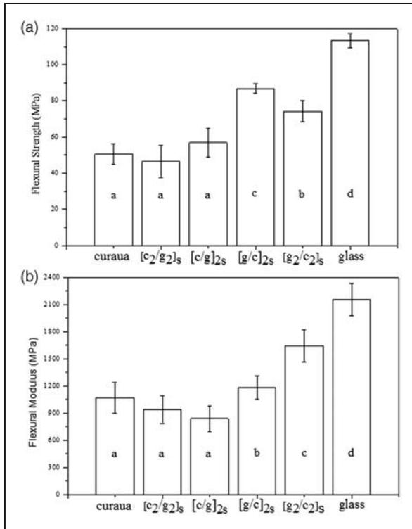
**Figure 2.** Mean values of flexural strength (a) and modulus (b) of the laminates.
