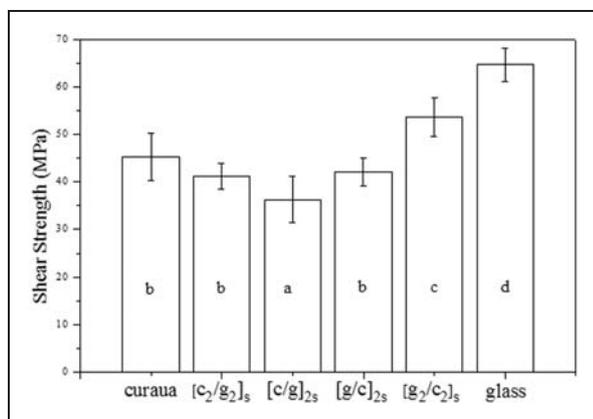
**Figure 5.** Mean values of Iosipescu shear strength of the laminates.
