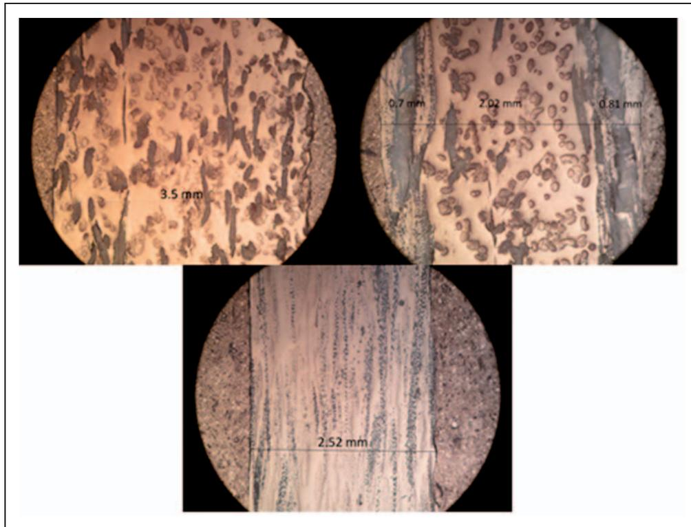
**Figure 1.** Optical microscopy of the laminates: (a) curaua, (b)  $[g_2/c_2]_s$  and (c) glass.
