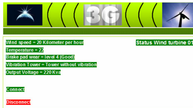
Figure 7. Monitoring and control system.
