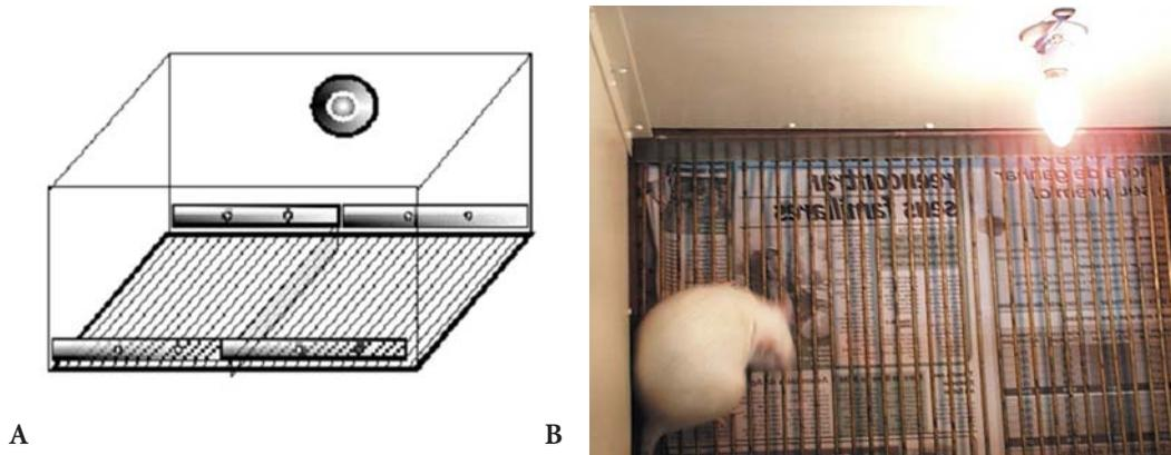
**FIGURA 7** – A) The Active Avoidance apparatus, also known as the Shuttle-box, resembles an IA box; only without the platform; each half of the grid is separated by a plastic hurdle and is independently electrified in order to deliver (B) the aversive stimulus – a footshock – according to the tone and the side in which the animal stands (two-way AA protocol).
